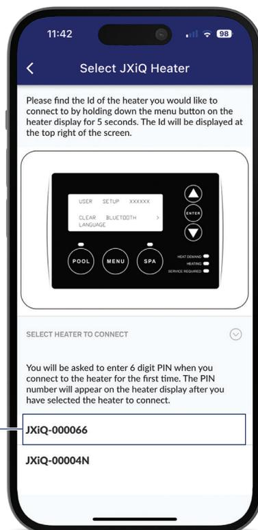
7. You will be asked to enter a **6-digit PIN** when you connect to the heater for the first time. 8. To get the **PIN** number, hold down the **“MENU”** button on the heater’s digital display for 5 seconds
